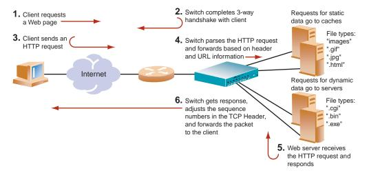
Figure 15-1 Content Intelligent Load Balancing Example
